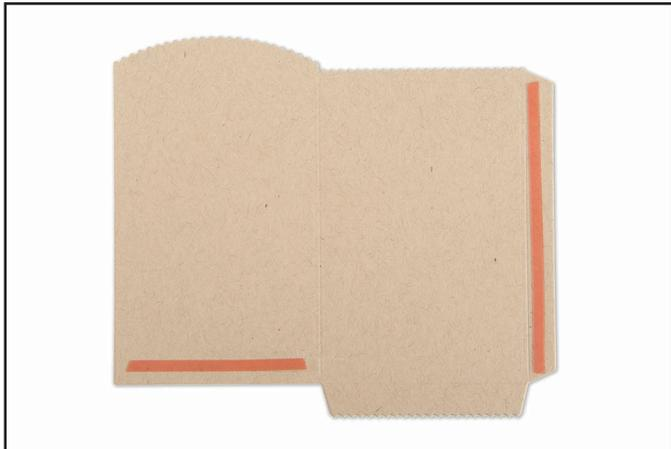
1. Die-cut out of desired material, and apply adhesive to the finished side along the bottom of the back panel and along the side tab.
