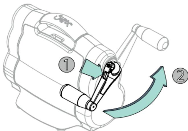
To begin using the machine, (1) press the lever in on the crank shaft to release the handle. (2) Lift the handle up vertically and pull it down so that it is parallel with the machine. The crank shaft will lock in place once it is in position. To store away, press the lever to release the handle from the locked position and twist up and down in front of the machine to lock in place.
