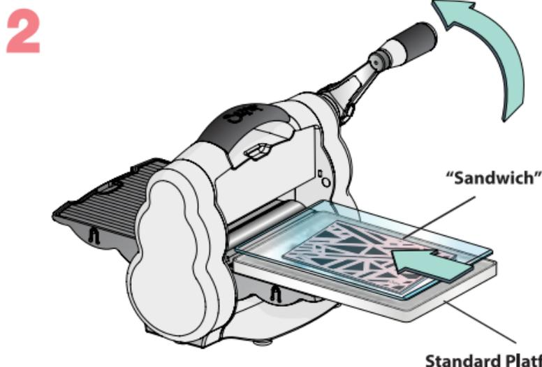
3. Place "sandwich" on Standard Platform and slide Platform into opening of Big Shot Foldaway. Note the rotation of the handle and continue to rotate it in the same direction until the Platform has passed through the opening and the rollers. Remove Platform from Big Shot Foldaway. Your embossed material is ready to use!
