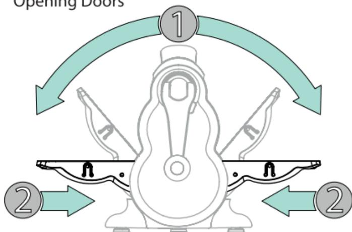
To open the machine, (1) pull down the beds from the centre using the finger grooves as a guide. (2) Once horizontal, push both beds in toward the centre of the machine to lock in place. To fold away, pull beds away from the centre using the finger grooves on the beds for grip. Once unlocked, fold beds up.
