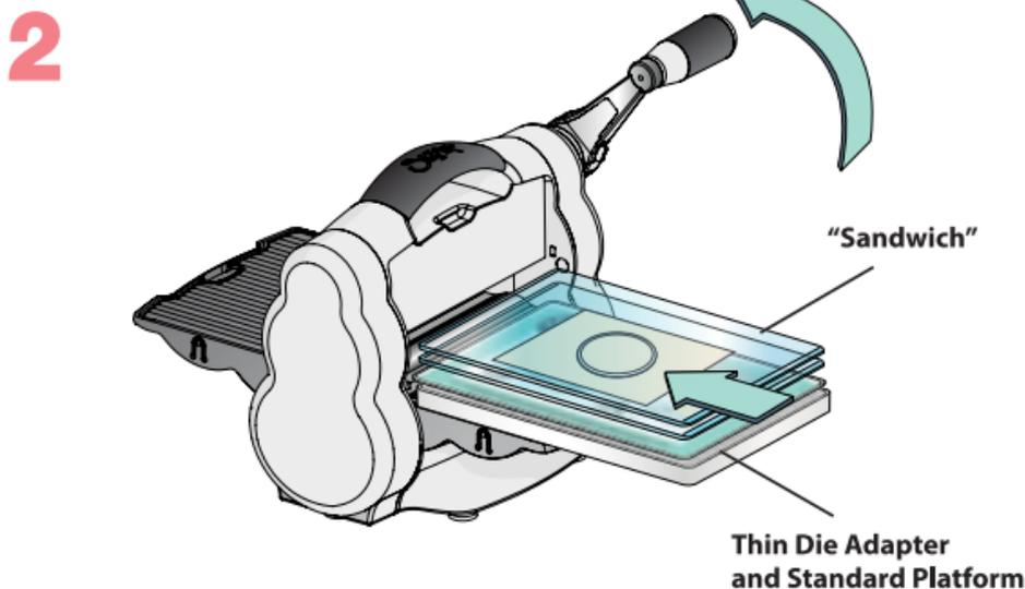
2. Place "sandwich" on both Thin Die Adapter and Standard Platform and slide platform into opening of Big Shot Foldaway. Note the rotation of the handle and continue to rotate it in the same direction until the Platform has passed through the opening and the rollers. Remove Platform from Big Shot Foldaway. Your die-cut shape is ready to use!
