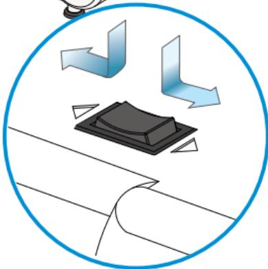
To operate the machine, gently depress the motor switch by pushing hardest on the side of the switch that points to the desired direction of the cut. Release all pressure from the switch and the rollers will stop moving. (Note: The machine moves in forward and reverse, allowing for reversal of direction at any time. This also makes for convenient loading and handling of shape-cutting products from either end of your Big Shot Express.)
