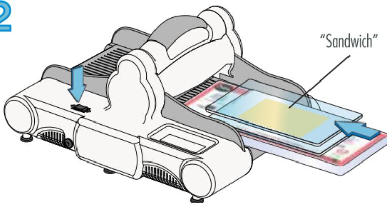
\* Insert sandwich and run through machine as directed.
