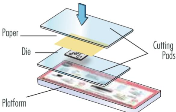
Place Sizzlits Die onto a Cutting Pad with foam side up. Place paper over the die. Place another Cutting Pad over the paper to create a "sandwich." For Clearlits Die, place die over photo or material so that the area to be cut shows through the die. Then place photo or material and die between Cutting Pads to make sandwich. Place "sandwich" on the platform.
